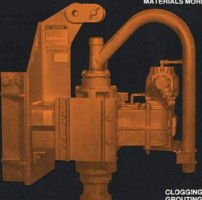
CLOGGING REDUCED WHEN GROUTING BY BUILT-IN ROTARY JOINT WITH 3 INCH I.D. KEEPS GROUT FLOWING.
